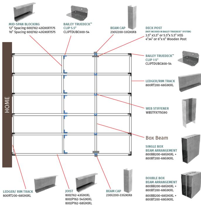
\*Position of the beam varies based on the position of the posts
